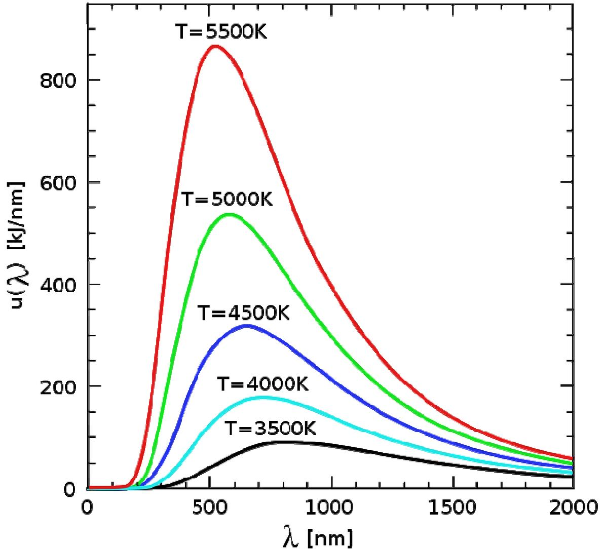
Figure 2. The distribution law for different T temperatures
