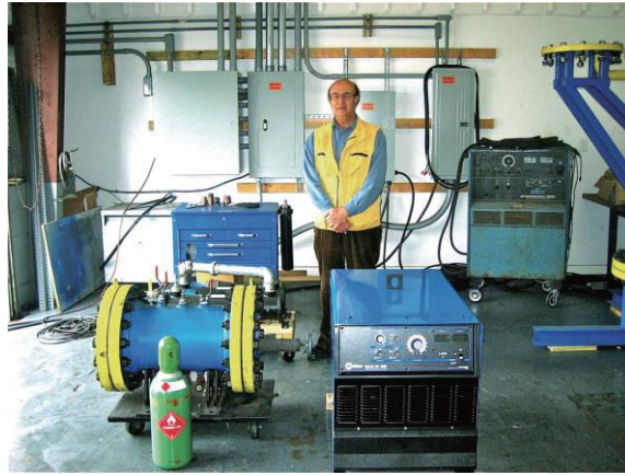
FIG. 3. Second reactor constructed with schedule 40 steel used in tests with hydrogen gas at 100 psi. [16] (Santilli, 2014). (Used with permission of Ruggero Santilli/Journal of Computational Methods in Sciences and Engineering)
