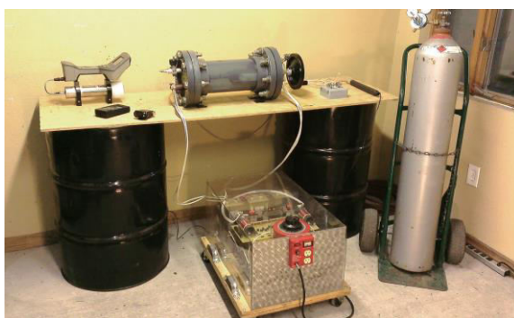
FIG. 4. One experimental setup, equipment from the left: SAM 940 neutron and gamma detector; a Polimaster, a Berkeley Nucleonics PalmRad; and a Ludlum neutron and gamma detector (not shown in this figure); the reactor; the specially built rapid DC pulsing power unit (patent pending) with incorporated capacitors in it; and the hydrogen bottle. [16] (Santilli, 2014). (Used with permission of Ruggero Santilli/Journal of Computational Methods in Sciences and Engineering)
