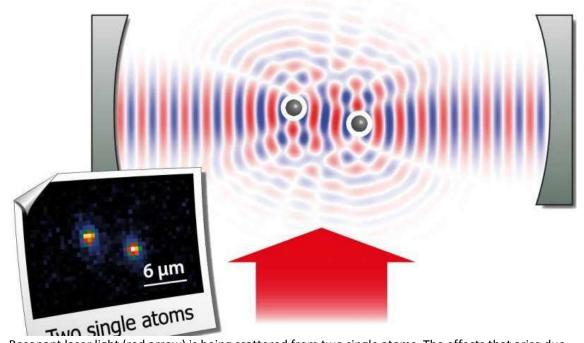
Resonant laser light (red arrow) is being scattered from two single atoms. The effects that arise due to interference (here shown in an artist's view) are determined by the relative spatial phase of the atoms and the interaction with the light mode of the optical resonator (mirrors in grey). Lower left: fluorescence image of two rubidium atoms. Credit: Andreas Neuzner, MPQ
