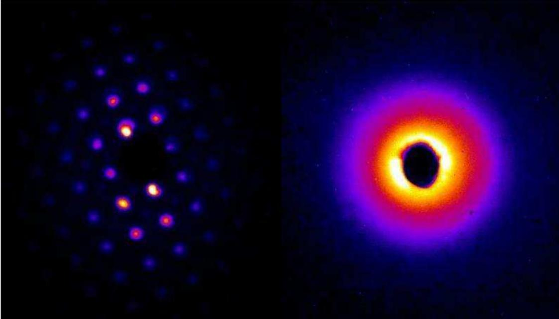
Ultrafast electron diffraction patterns of single-crystal gold (left) and nitrogen gas (right) obtained with SLAC's new experimental setup. By analyzing changes in patterns like these, scientists learn about motions in materials that take ...more
