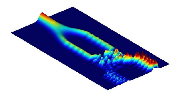
Interferometry: A beam is split into two parts, which are then rejoined. From the way in which the two beams interfere; one can deduce which forces acted on the beams. Image source: TU Wien http://www.tuwien.ac.at/dle/pr/aktuelles/downloads/2013/quantenrauschen/
