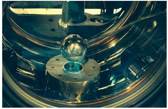
A vacuum chamber with a marble-size sphere at its center was used to test the nature of dark energy.
